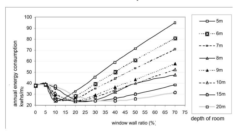
Optimum area of glazing in sub-tropical climates is less than temperate climates
