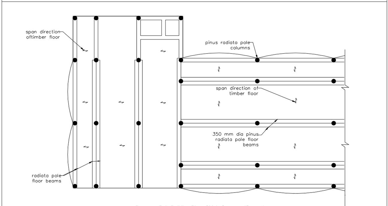
Prototype Pole Building-Plan of Main Structure (figure 5)
