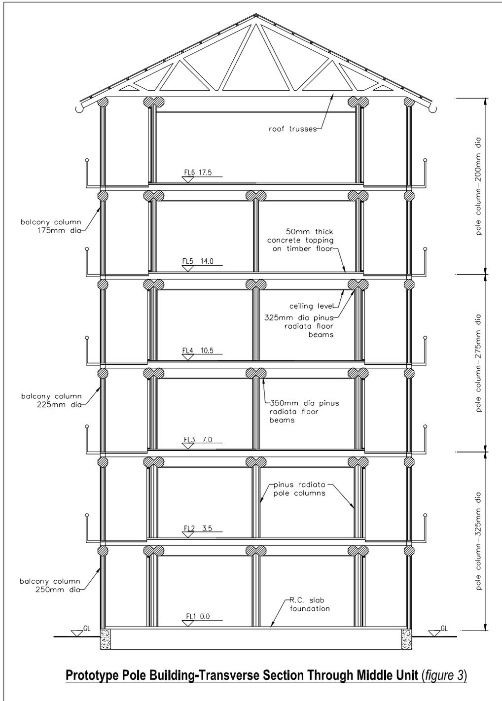
The main structural elements were radiata pole floor beams, radiata pole columns, timber floors, and plywood wall diaphragms. The pole elements formed a simple post-beam system. The party walls were designed as plywood sheathed diaphragms to resist wind and earthquake loads.
