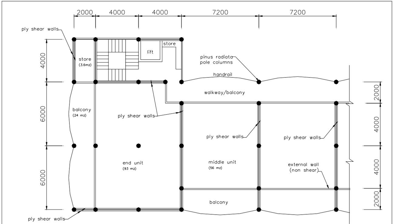
Prototype Pole Building-Plan of Units (figure 1)
