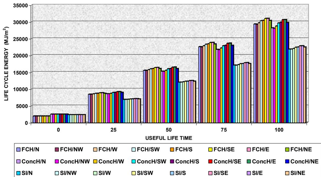
Fig. 3: Comparison of impact of orientation and construction type on heating energy use in Christchurch with whole day heating
