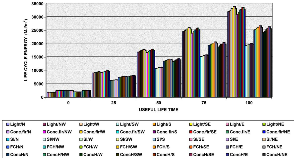
Fig. 2: Comparison of impact of orientation and construction type on the energy use in Wellington with whole day heating
