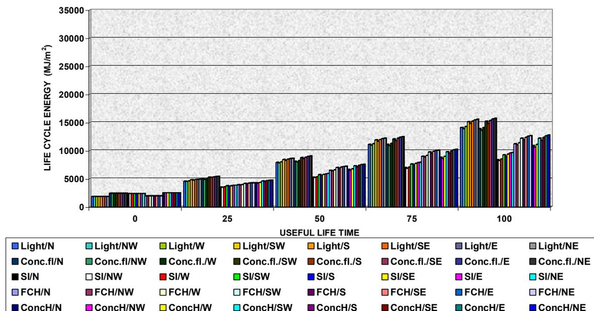
Fig. 4: Comparison of heating energy requirement for various construction types with intermittent heating in Auckland
