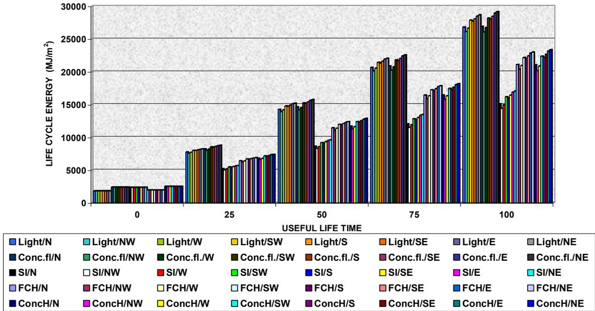
Fig. 5: Comparison of heating energy requirement with intermittent heating for various construction types in Wellington
