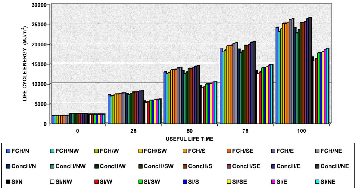
Fig. 6: Comparison of heating energy requirement with intermittent heating for various construction types in Christchurch
