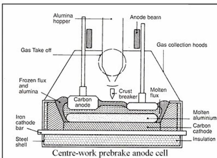
Figure 1: Cross Section of Reduction cell.
