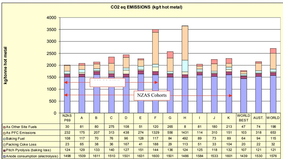
Figure 3: CO<sub>2</sub> emissions from NZAS compared with other smelters.
