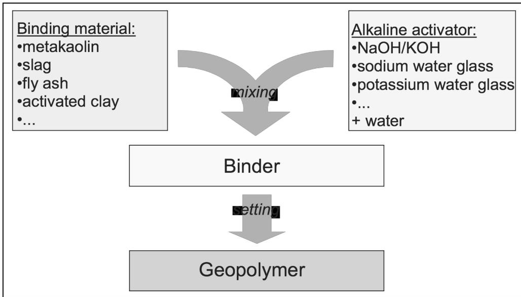
Figure 2: Production of the geopolymer
