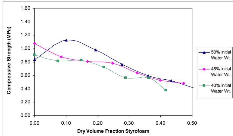
Figure 1: Average strength vs. polystyrene content (separated by water content)
