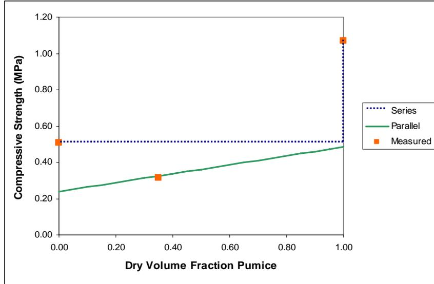
Figure 6. Load sharing behavior of Ohaaki clay / pumice composite
