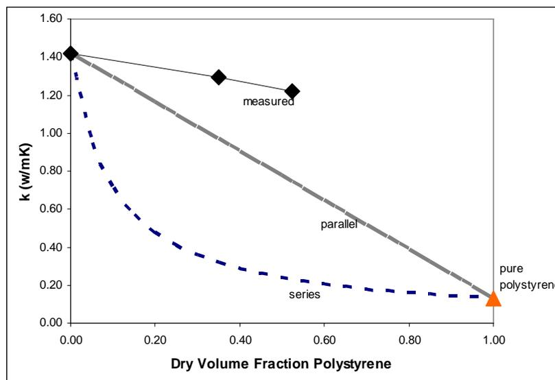
Figure 4: Thermal modeling of polystyrene composite
