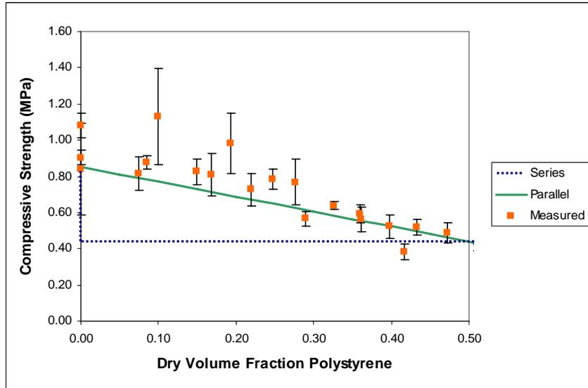
Figure 5: Load sharing behavior of polystyrene composite
