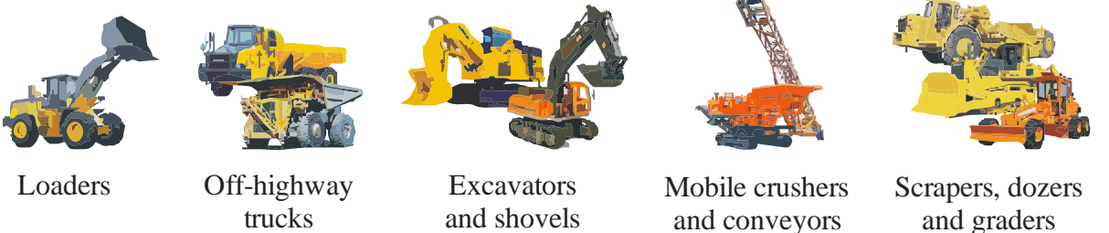
Figure 5: Some examples of construction and mining equipment
