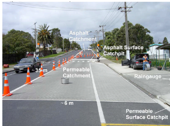
FIGURE 3: PERMEABLE PAVEMENT EXPERIMENTAL SECTION ON BIRKDALE ROAD
