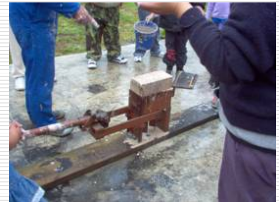
Cinva ram brick fabrication on-site in Te Toke NZ - photos courtesy of Bryan Innes
