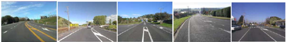
Figure 4 – Non self-explaining roads, with posted speeds of 100, 80, 70, 60 & 50 km/hr, but all giving similar perceptual cues
