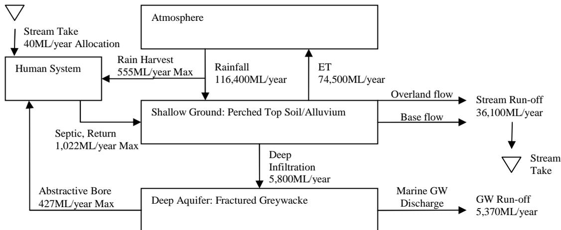
**Figure 4. Conceptual Model and Component Scale.** GW=groundwater.
