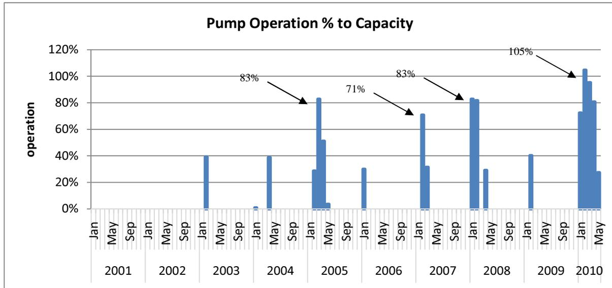
**Figure 5. Seasonal Operation of Pumps.** Monthly bore water supplement required was calculated from daily-step rain-harvest-pump simulation and divided by the current island-wide instantaneous pump rate capacity of 427ML/year. The island-wide pumps were frequently running at risky levels of reaching the capacity cap in many summer seasons and the pump capacity was finally breached in February 2010.
