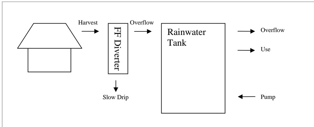
**Figure 1. Rainwater Harvesting Simulation Structure.** One-roof, two-tanks. The collected volume is first passed through the First Flush Diverter (FFD). The overflow of the FFD is stored in the main Rainwater Tank.
