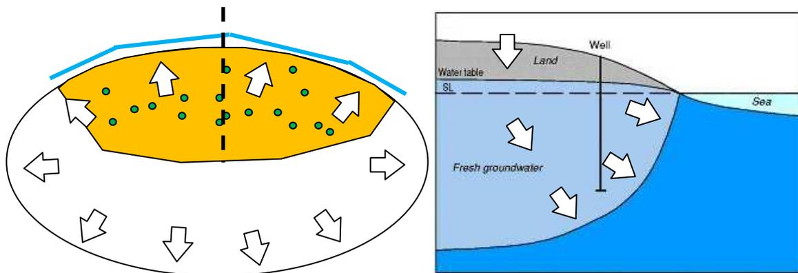
**Figure 7. (Left) Hydraulic Push on a Hypothetical Island and (Right) the Vertical Cross-Section.** Green dots represent bore pumps. Cross-section source: OzCoast (2010).
